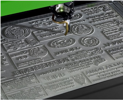
Engraving & laser cutting of custom ink stamps
