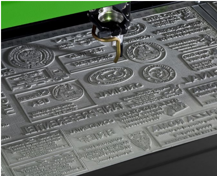
Engraving & laser cutting of custom ink stamps
