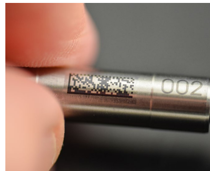
Annealing on stainless steel
