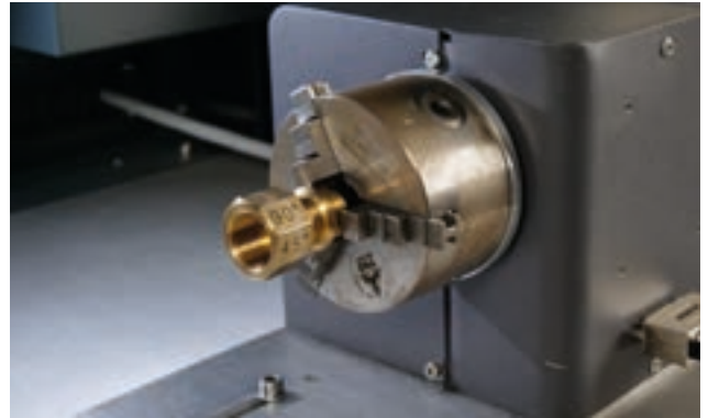
Engraving of cylindrical parts
