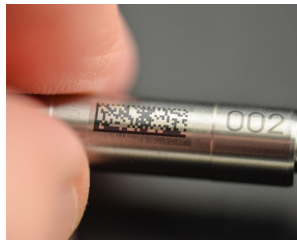
Annealing on stainless steel
