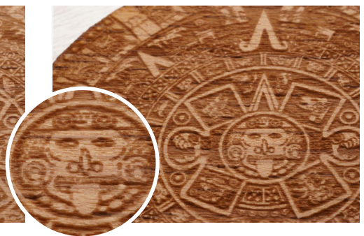
4.0" engraving A rough engraving that looks blurred
