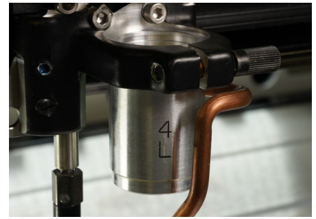
Lens 4.0" Thick cutting and fast engraving
