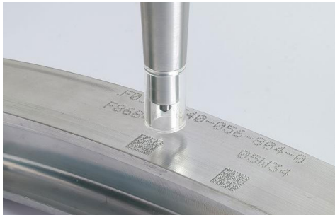
Electromagnetic dot peen stylus
